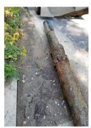
pipe is buried up to 9 ft. in the ground (too deep to safely maintain), and 3) cast iron pipe is not resilient to ground shifts and earthquakes.
