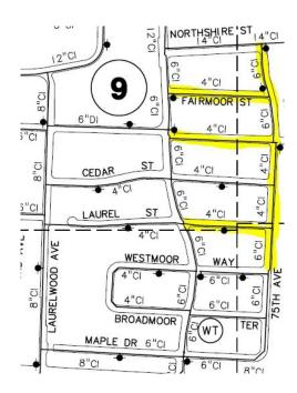
**Project Justification:** This project will replace a cast iron main installed in the late 1940s. The District has made
