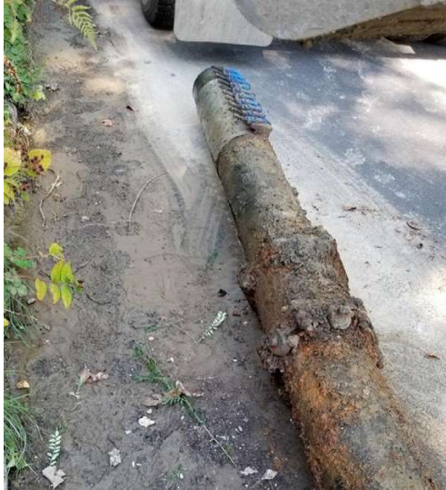
Garden View pipe that was replaced in 2022 shows extensive corrosion.
